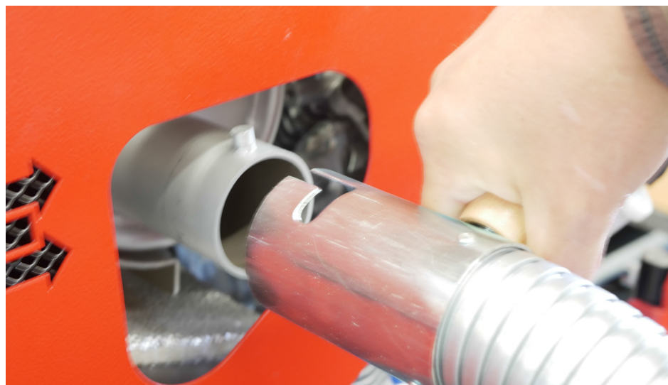
Fig. 8-5 Connecting up the exhaust hose
